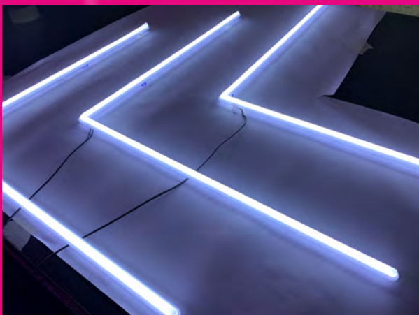
LED neon built into 10mm white acrylic. Used as individual wayfinding arrows complete with plastic stand off fixings to rear and paper template for fixing.
